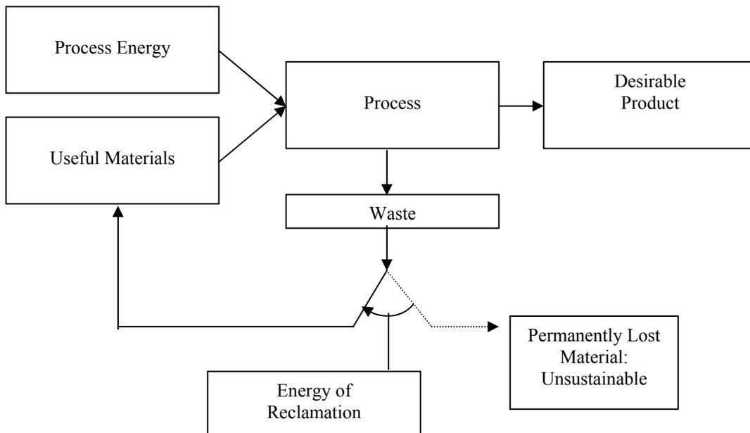
Figure 1. Sustainability is a function of the energy of reclamation needed to make the percentage of Permanently Lost Material smaller than some specified value.
